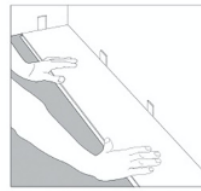
1. Begin installation from left to right. Install spacers at ends & where planks meet wall.
